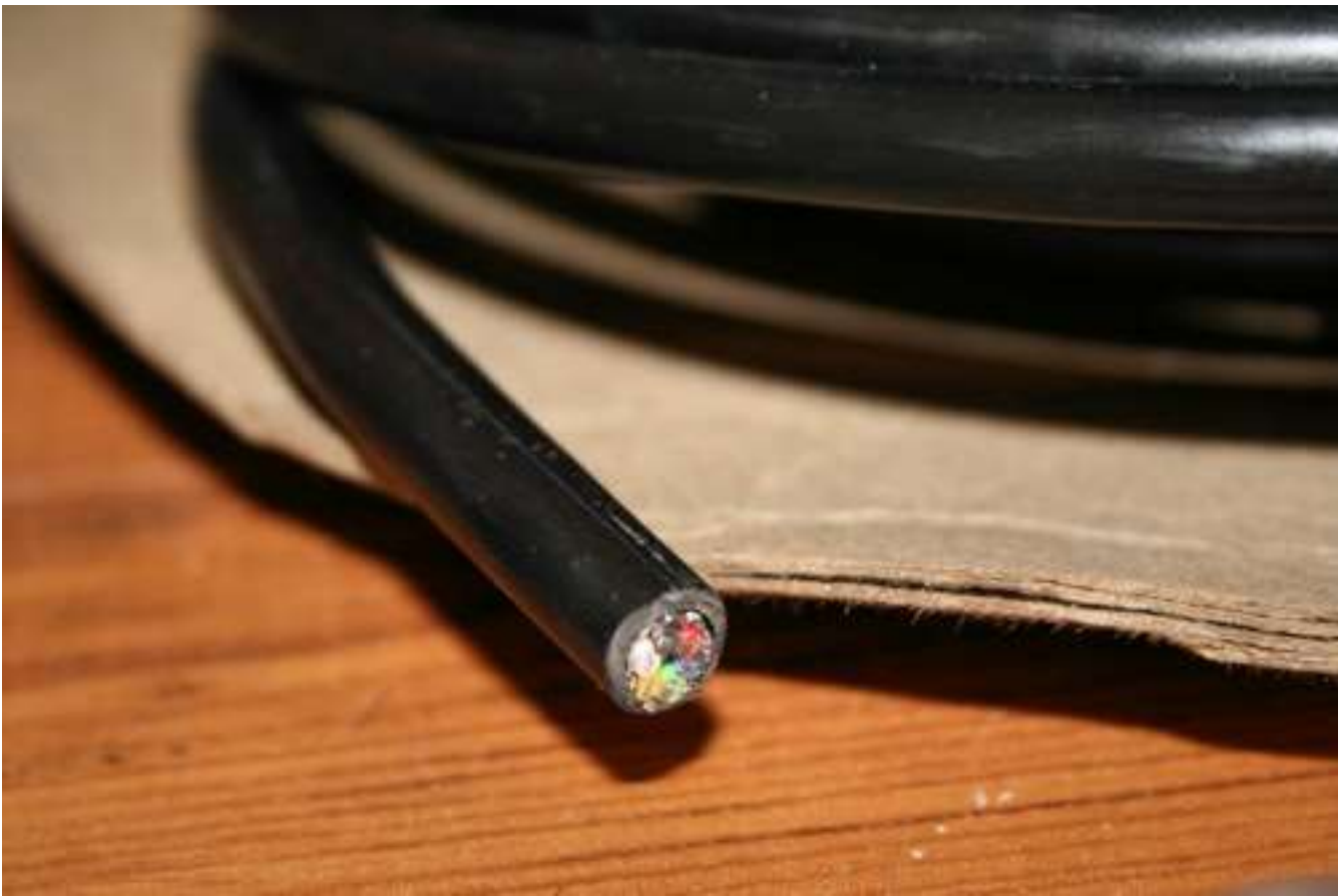
This is a close-up of the shielded video cable. This particular cable is Defstan 6 Multi-Core Cable, 16/0.2 mm for each core. It is a specialised video cable used in the construction of SCART leads. It is quite expensive though, so whichever cable you choose to carry the video signal just make sure it has a braided shield/screen, otherwise you may get ghosting on your display.
