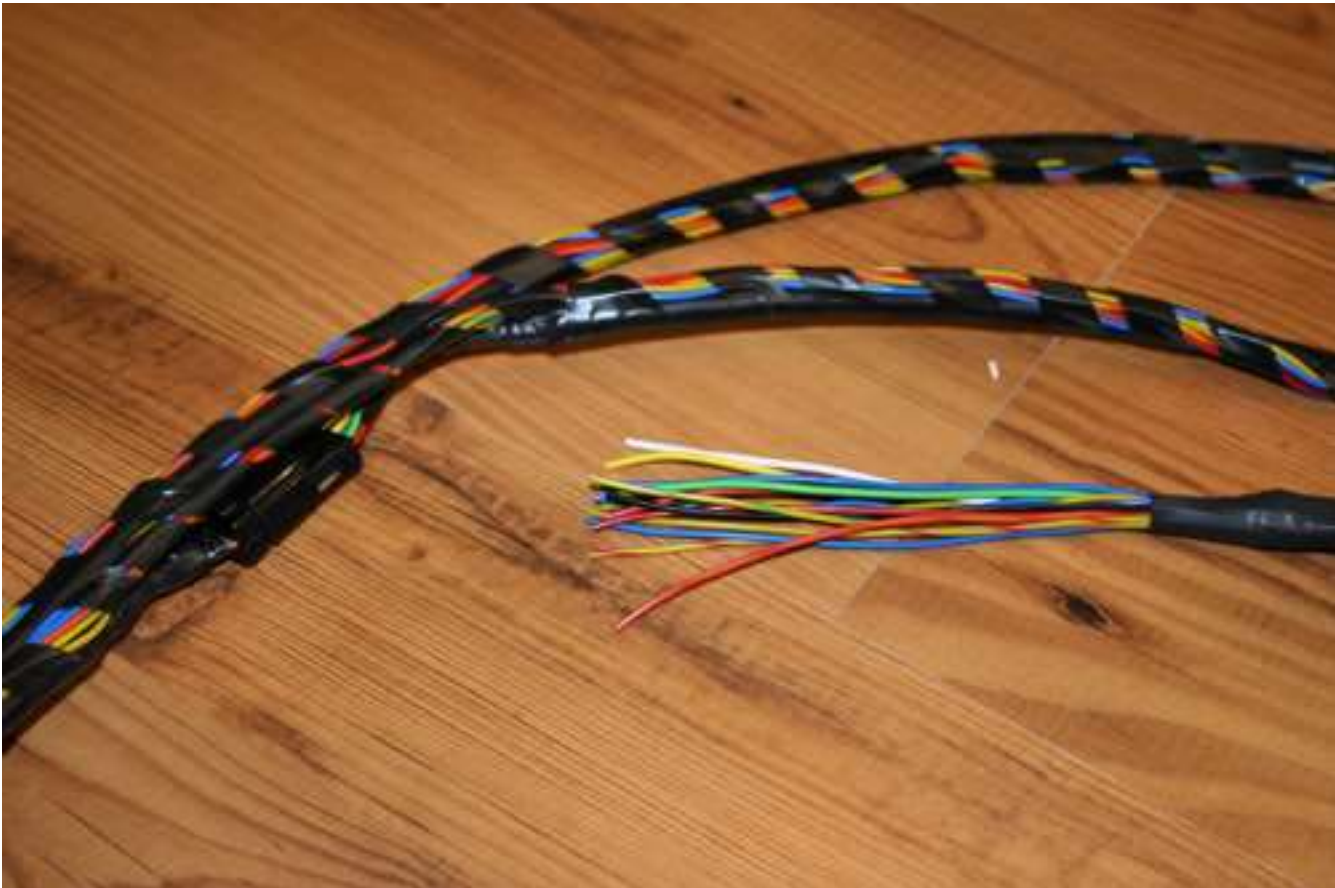
Using the schematic splice the cables together as appropriate using heat shrink solder joints.
